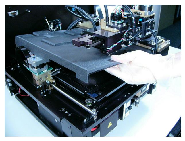
Figure 5-10: Removing the incubator housing
