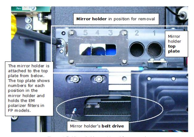
Figure 4-5: Mirror holder positioned for removal
