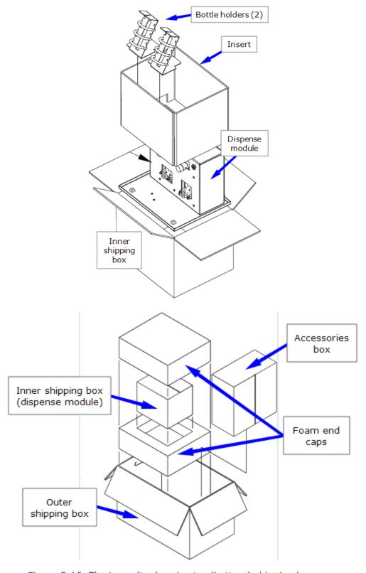
Figure 2-16: The inner (top) and outer (bottom) shipping boxes
