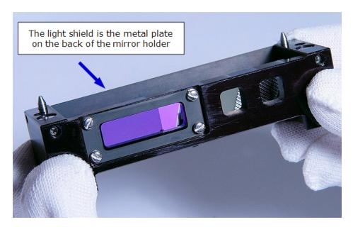
Figure 4-7: Mirror holder removed from reader
