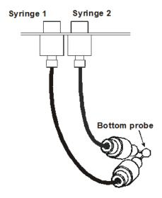
Figure 3-6: Injectors inside the reader
