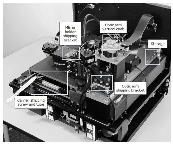
Figure 2-4: Internal compartment, with shipping hardware
