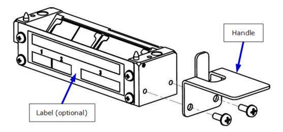
Figure 4-12: Attaching the handle to the mirror block
