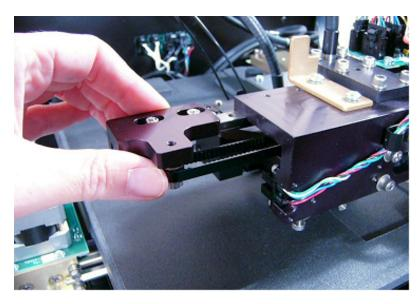
Figure 4-6: Turning the belt drive to position the holder for removal
