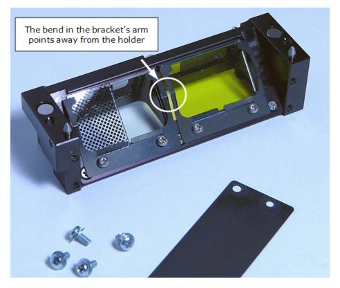
Figure 4-10: Mirror holder with shield removed
