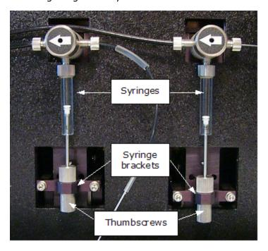
Figure 2-13: Dispense module, close-up view of syringes
