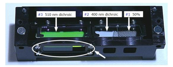
Figure 3-4: Identifying the mirrors in the mirror holder (default configuration shown). Models with the Fluorescence Polarization module also have EX polarizing filters in the mirror holder, as shown inside the oval above.
