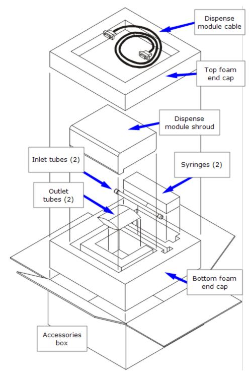
Figure 2-15: Packing the dispense module accessories
