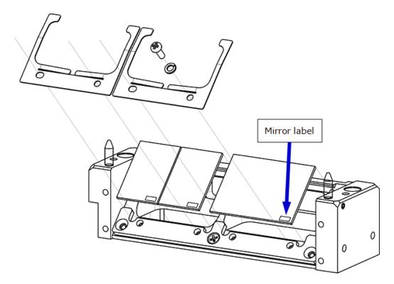
Figure 4-9: Mirror orientation; labels are face-up and readable
