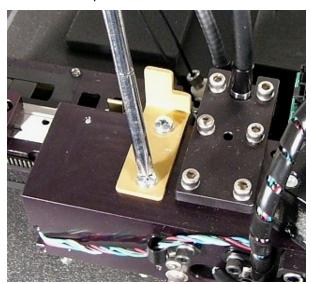
Figure 2-9: Mirror holder shipping bracket, in its storage position
