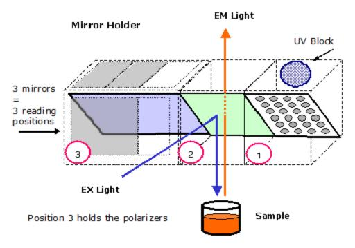
Figure 4-3: Mirror holder diagram; the three reading positions are indicated
