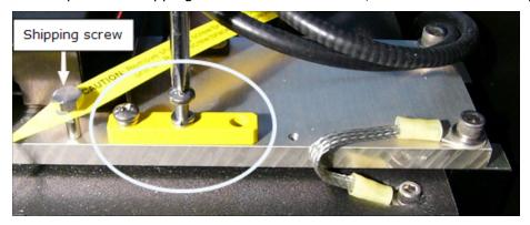
Figure 2-7: Carrier shipping screw and optic arm shipping block stored on the base plate
