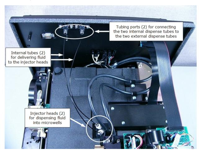
Figure 5-1: Internal components for the injection system
