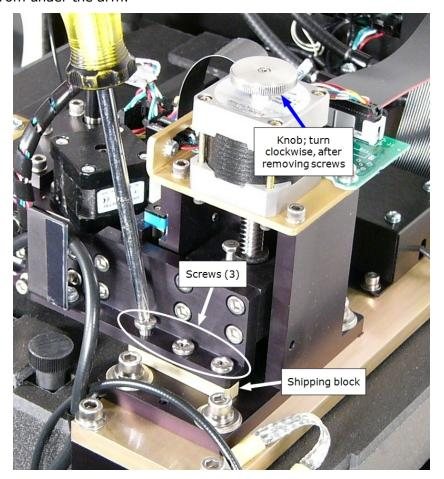
Figure 2-6: Removing the optic arm shipping block
