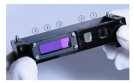
Figure 4-2: Mirror holder disengaged from the reader
