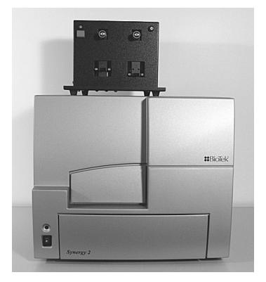
Figure 2-11: Dispense module on top of the reader
