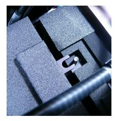
Figure 5-12: Positioning the incubator housing fork
