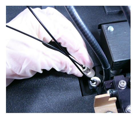
Figure 5-3: Disconnecting the tubes from the injector heads
