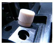
Figure 5-13: Seating the injector head
