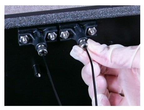
Figure 5-2: Disconnecting the dispense tubes from the back wall
