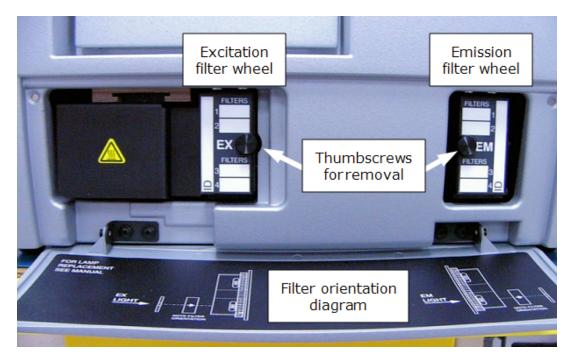
Figure 3-3: Locating the excitation and emission filter wheels
