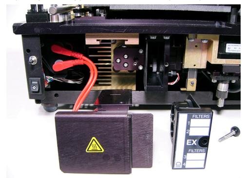
Figure 6-1: The light-blocking panel and excitation filter wheel removed for lamp replacement
