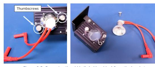
Figure 6-2: Removing the old bulb (with cables) from the bracket
