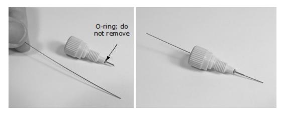
Figure 5-6: Using the stylus to clean an injector head
