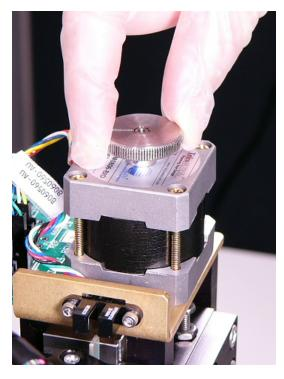
Figure 5-9: Raising the optics armature
