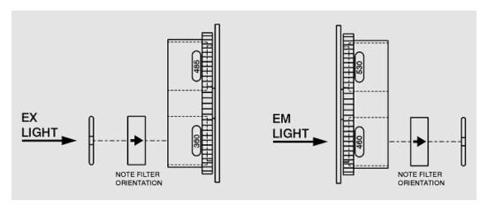
Figure 4-1: Diagram showing the proper orientation of the filters in their wheels
