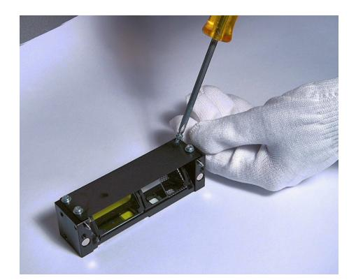
Figure 4-8: Removing the light shield from the mirror holder
