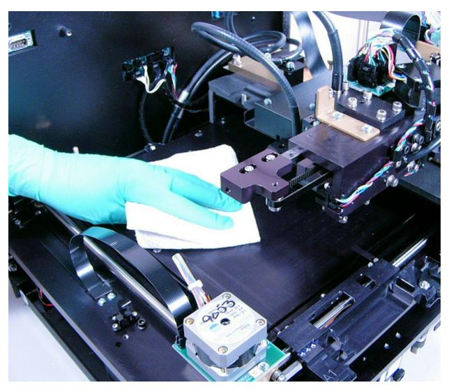
Figure 5-11: Cleaning the inside of the reader
