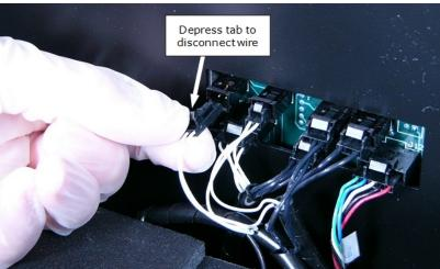
Figure 5-8: Disconnecting heater wires 1 and 3 in the top row
