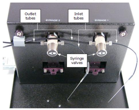
Figure 2-12: Dispense module components
