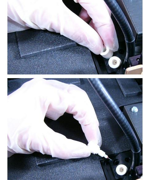
Figure 5-4: Removing the injector heads
