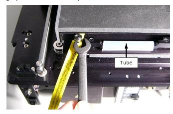
Figure 2-5: Removing the carrier shipping screw and tube
