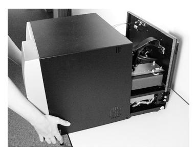
Figure 2-3: Sliding off the shroud
