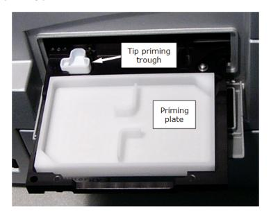
Figure 2-14: Priming trough and plate installed on the carrier
