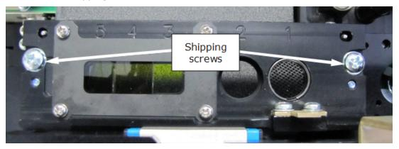
Figure 2-10: Mirror holder shipping screws
