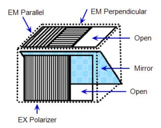
Figure 4-4: Mirror holder, Position 3 diagram
