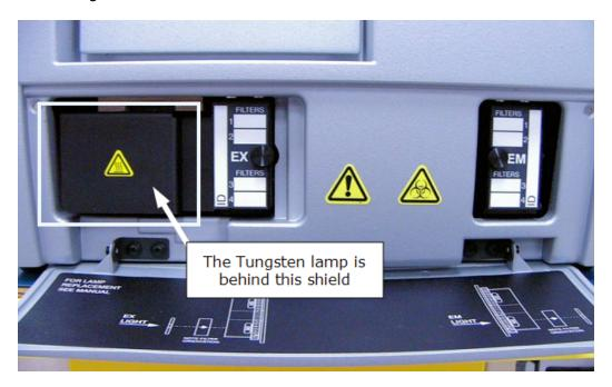
Figure 3-2: Locating the replaceable Tungsten lamp
