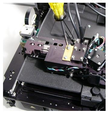
Figure 2-8: Removing the mirror holder shipping bracket
