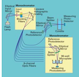
The SpectraMax Reader's optical system mimics a dual-beam spectrophotometer. Each sample has a discrete sample beam and reference beam.
