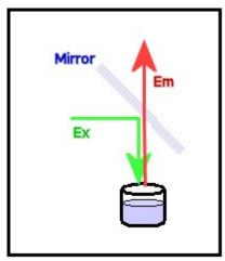
**Dichroic mirrors have to match the Excitation and Emission filters**. If the excitation filter and dichroic do not match, the excitation light goes through the mirror, instead of reflected to the sample and the sample does not get excited. If the emission filter and dichroic don't match, even when the excitation light is reflected to excite the sample, the emission light is also reflected by the mirror and goes back to the light source instead of the detector (PMT).
