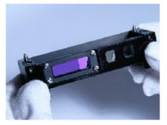
Mirrors reside in a mirror holder with three possible reading positions. Any mirror can be used for any type of experiment, except FP (Fluorescence Polarization), which
