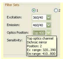
In the Read Step dialog, hover your mouse over the **Optics Position** to see a tool-tip that lists the Excitation and Emission range for the selected dichroic mirror. Either select filters that fall within the Ex and Em ranges (respectively) or change the selected mirror.
