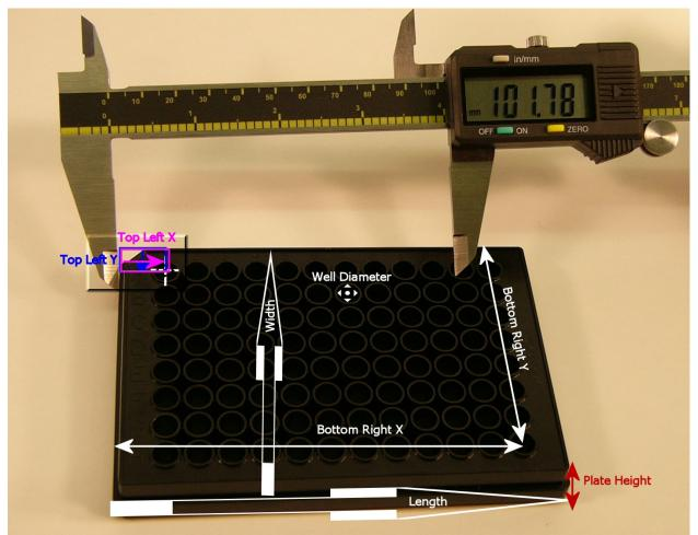
When creating or updating plate dimensions, taking precise measurements is essential. Use calipers with precision to 0.01 millimeters (mm) to gather the following measurements. A standard ruler is not precise enough. Note: when entering values based in 10 micron increments, values always end in 0 (zero).
