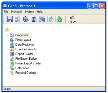
The workspace is made up of the menu tree with a branch for each of the protocol's elements. The order of the protocol elements reflects the order to follow when defining most protocols:
